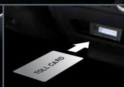
Built-in Toll Reader
